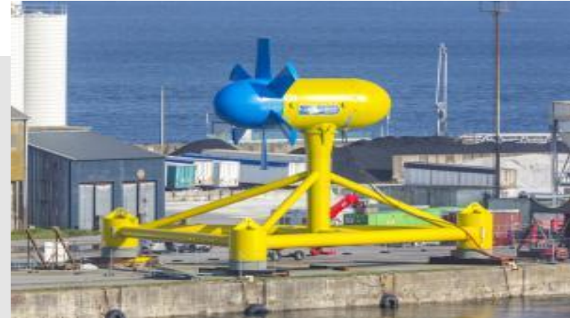
Hydrolienne SABELA D10 (250 kW) 100 % made in France (Ouessant)
